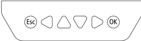
The buttons are respectively (from left to right) "ESC", "Left", "Up", "Down", "Right" and "OK" buttons, the operation is described in the schematic operation diagram below:
