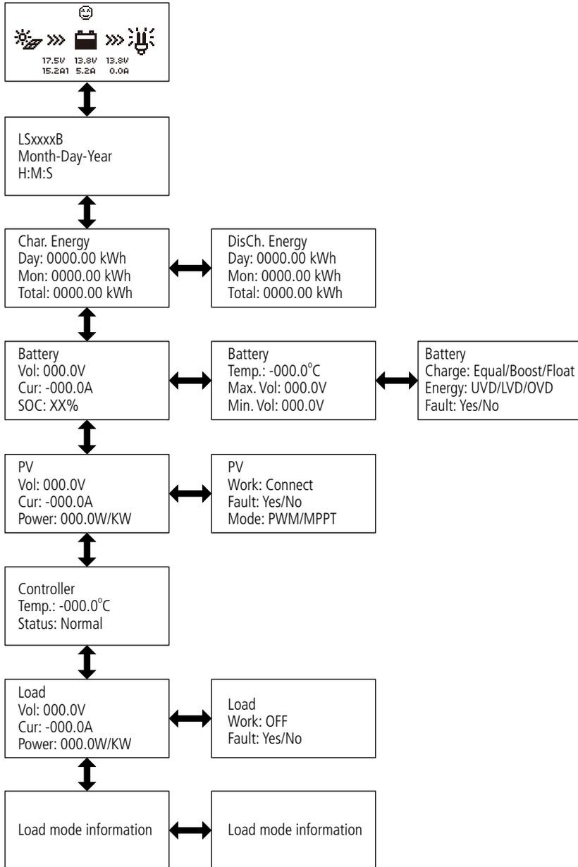
**Operational tips:**  $\triangle$  and  $\nabla$  buttons are respectively used to turn the browse page upward and downward, while  $\triangleleft$  and  $\triangleright$  buttons are respectively used to turn the interfaces left and right.
