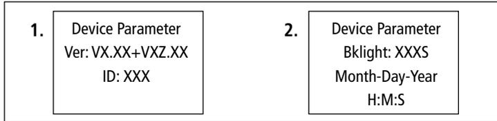
**Note:** the bigger the ID value of the connection device, the longer the Meter communication identification interval (the maximum interval<6 minutes).
