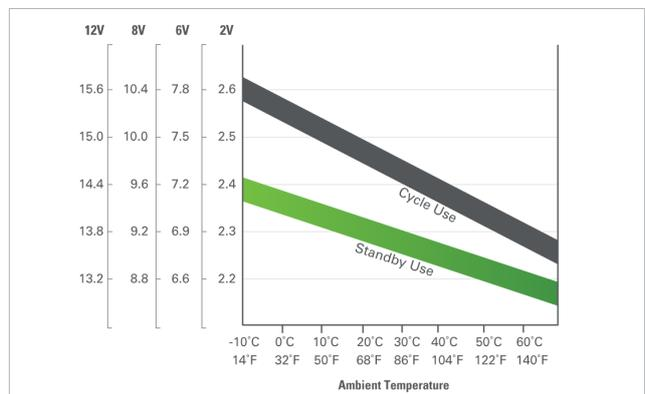
1. Due to self-discharge characteristics of lead-acid battery technologies, batteries should be top charged within 6 months of storage to ensure optimum performance, prevent sulphation and permanent capacity loss.
