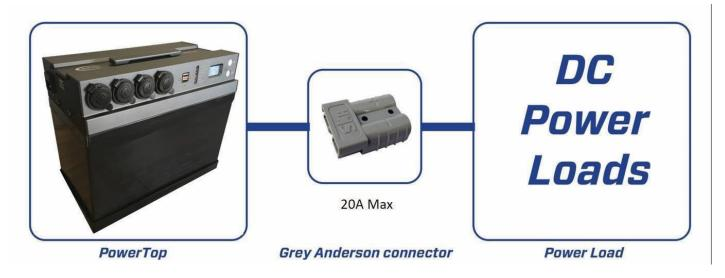
Loads can also be connected to the following 12V DC Power sockets:
