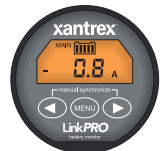
AMPS Net charge or discharge current going into or out of the battery bank
