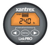
TIME REMAINING Time remaining in hours & mins until deepest discharge threshold reached
