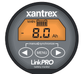
AMPERE HOURS Counts and displays the amount of ampere hours removed from the battery (up to 9999Ah)
