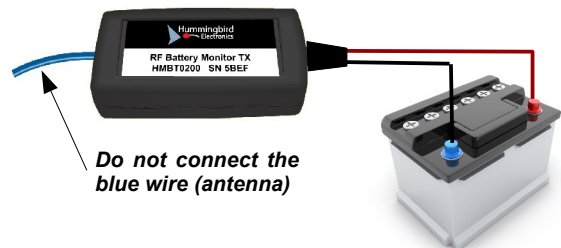
Wire the transmitters directly to the batteries to be monitored
